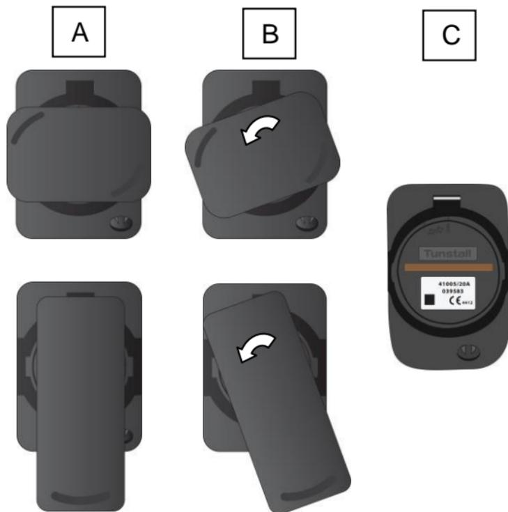
2) Remove the battery cover, insert a coin into the slot and turn it counter clockwise.
